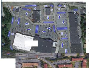
Develop a Site Engineering / Layout Plan: The manager or contractor should complete a pre-season site survey using a map of the property to determine property boundaries and physically stake the property, areas to be serviced, locations of hazards / obstacles, identify areas to relocate snow, determine the pattern or direction to best move snow as well as spread salt and other deicers.
